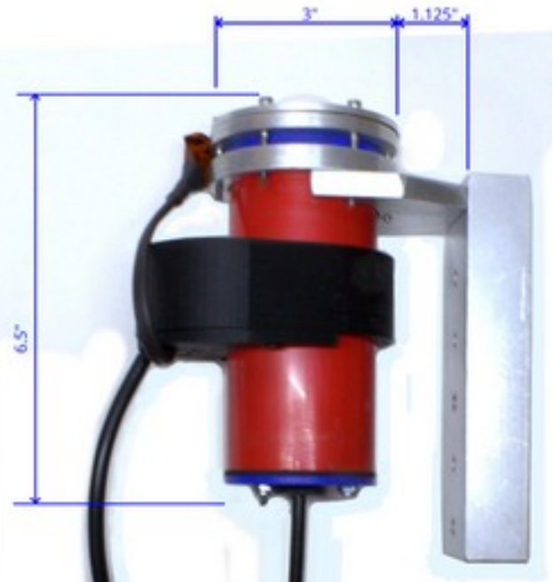
Figure 4: Astra180 USB camera dimensions.
