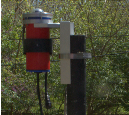
Figure 8: Astra180 Mounted on a \geq 1\ 7/8 " OD pole. Channel straddles the pole. Secured with hose clamp.
