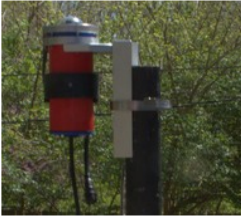
Figure 8: Astra180 Mounted on a \geq 1 \frac{7}{8} " OD pole. Channel straddles the pole. Secured with hose clamp.
