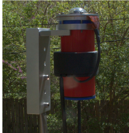
Figure 7: Astra180 mounted on < 1\ 7/8 " OD pole. Pole is inside channel.
