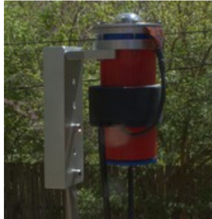
Figure 7: Astra180 mounted on < 1 \frac{7}{8} " OD pole. Pole is inside channel.
