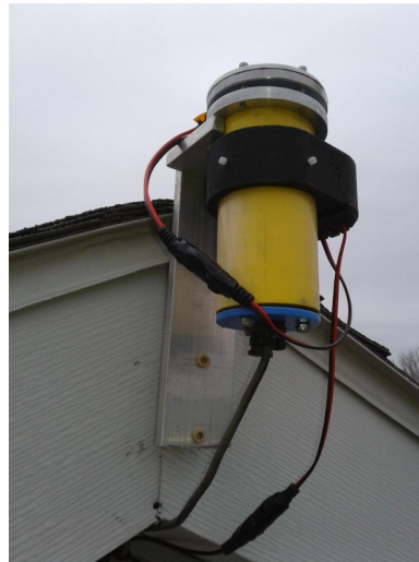
Figure 18: Camera mounted at the peak of a roof against the Fascia Board using a flat.
